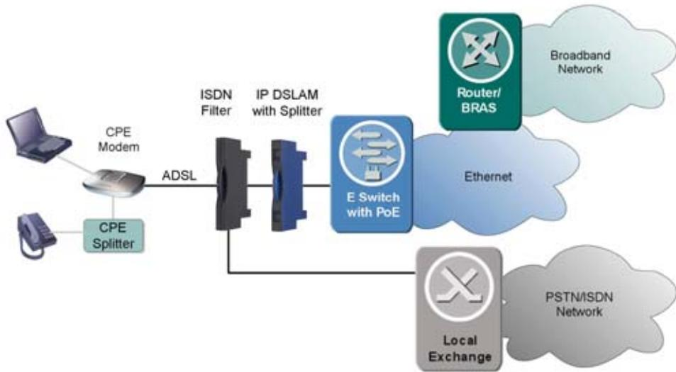
*Figure 51 Base band Solution with External ISDN Filter*
