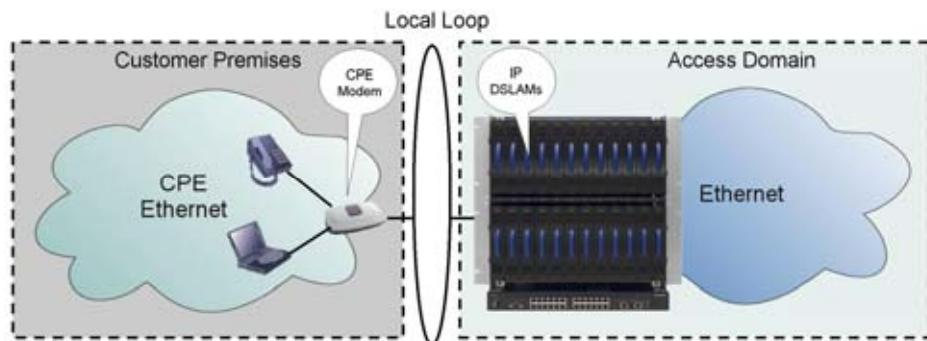
*Figure 7 Bridging the Access Domain and the CPE Ethernet*
