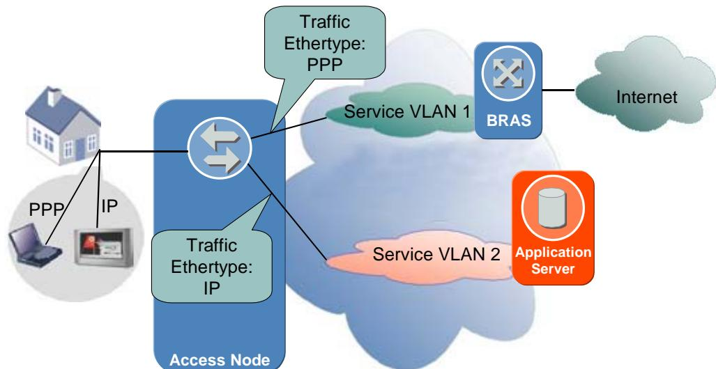
*Figure 33      Traffic Mapping to Two VLANs*
