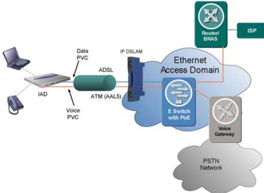
*Figure 52      Telephony over IP Architecture*
