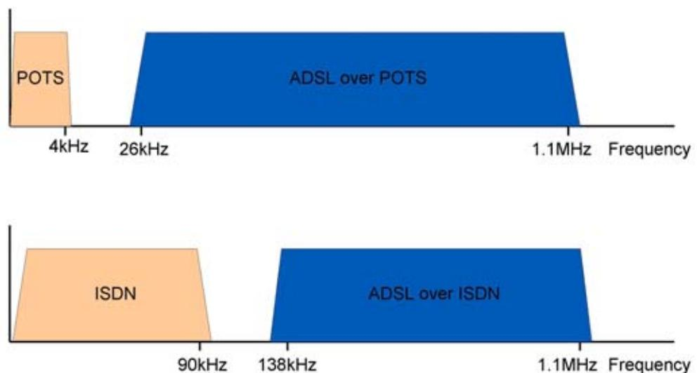
Figure 48      *Base band POTS and ISDN Frequency Separation*
