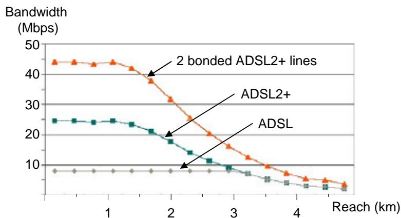
Figure 2      Line Bonding Utilization
