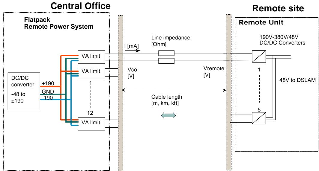
Figure 27 Block diagram for the remote powering
