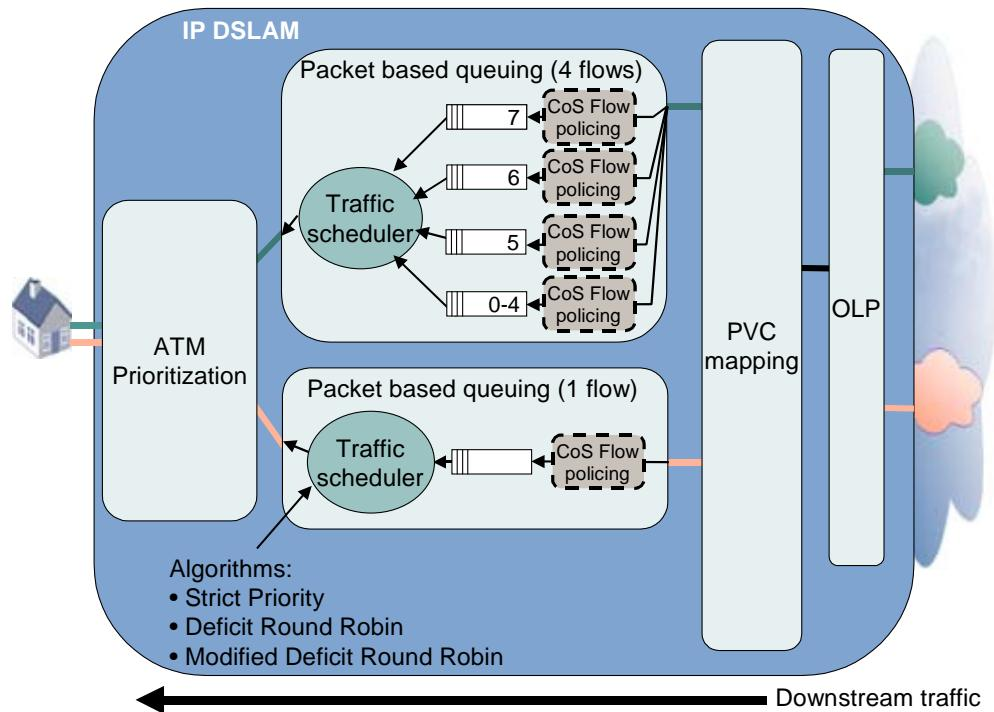
Figure 43 Packet Based Queuing
