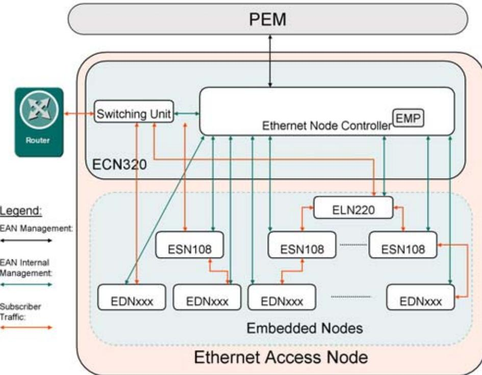
*Figure 15      Ethernet Access Node Structure*
