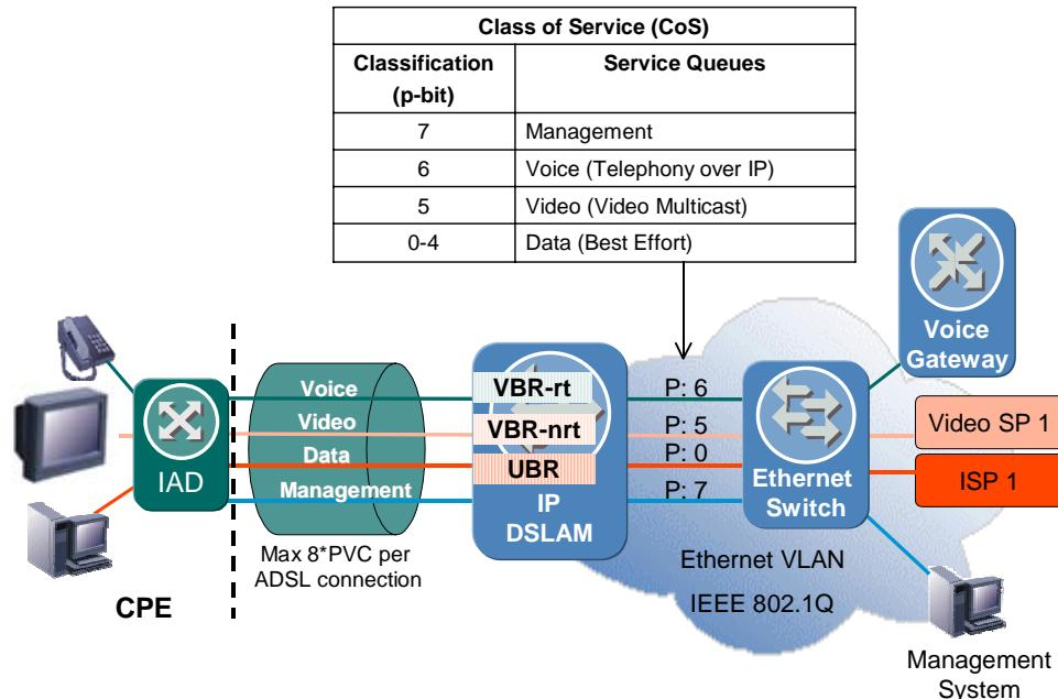
Figure 46 Service Mapping and QoS in EDA
