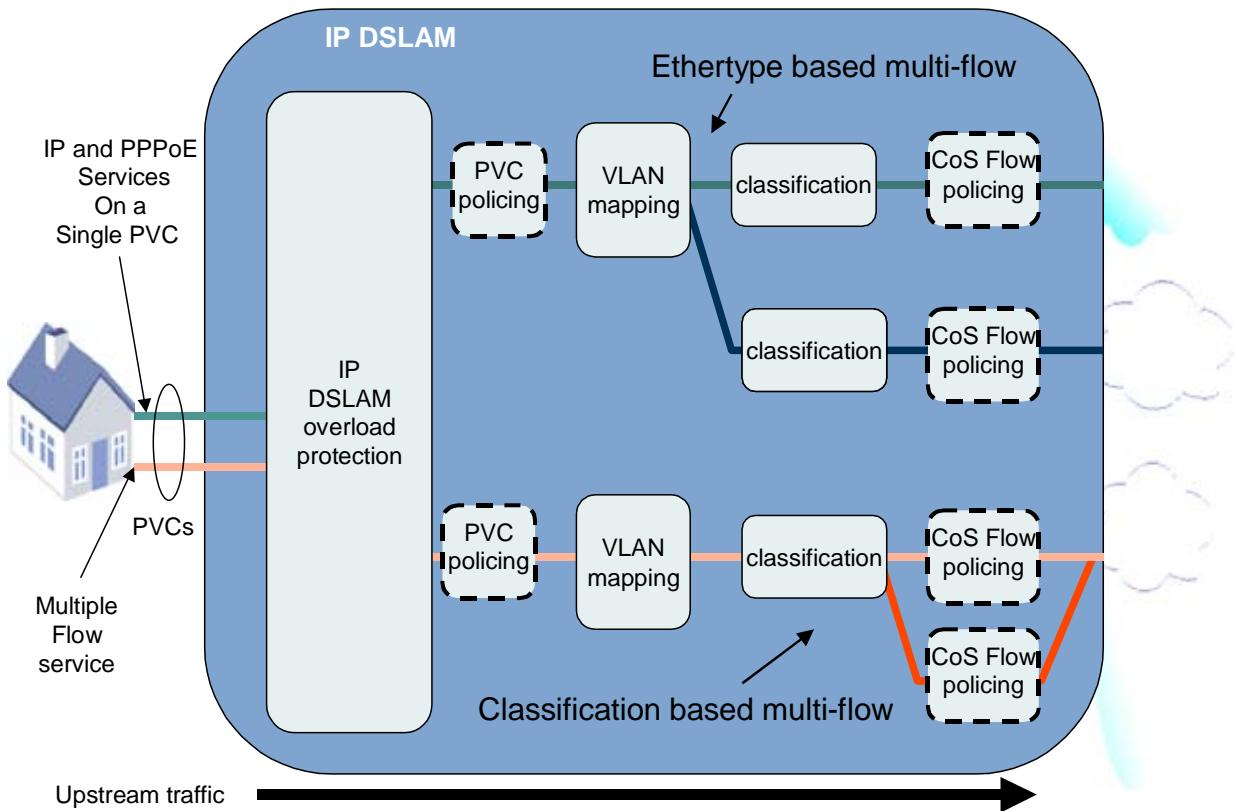
**Figure 47      Upstream QoS Mechanisms**
