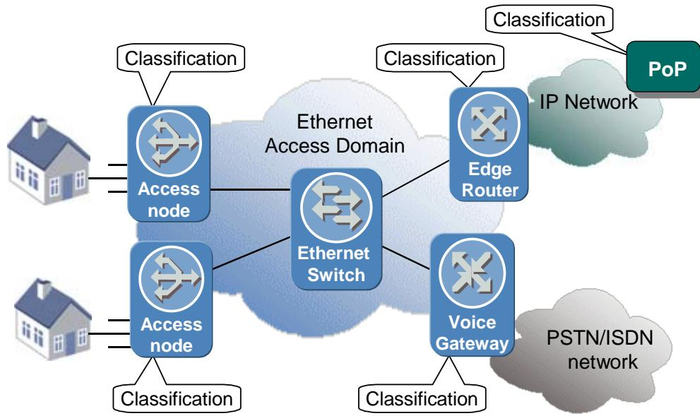
*Figure 38      Traffic Classification in an EDA Network*
