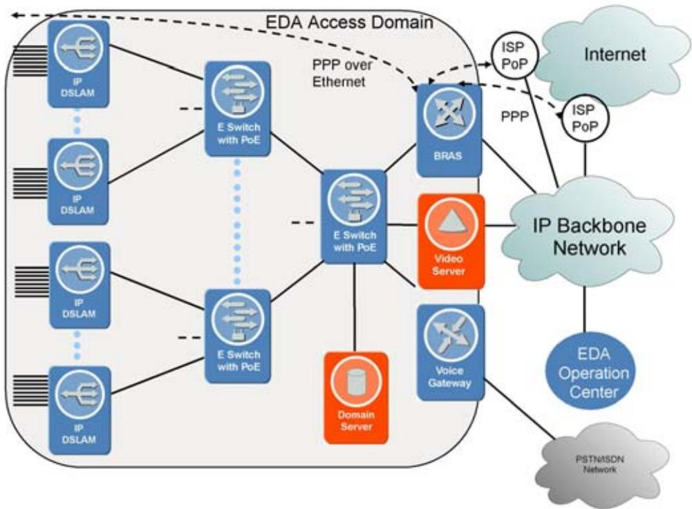
*Figure 61 EDA Access Network Incorporating a BRAS*
