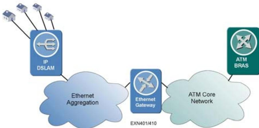
*Figure 26 Migration from Ethernet to ATM through EXN401/410*
