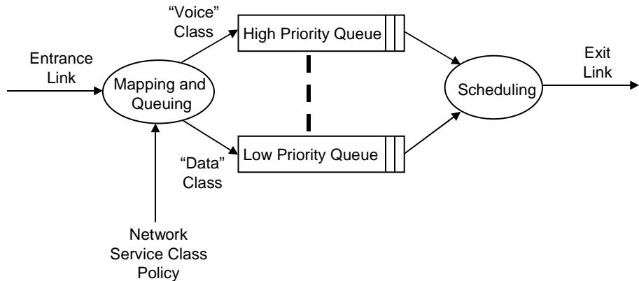
*Figure 39      Differentiated Services in an Ethernet Switch*
