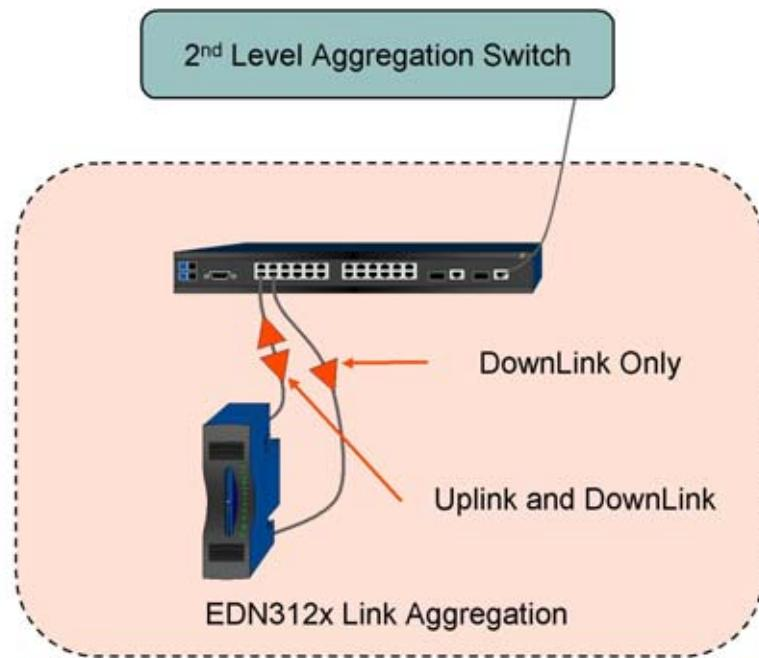
*Figure 12      EDN312 Link Aggregation*
