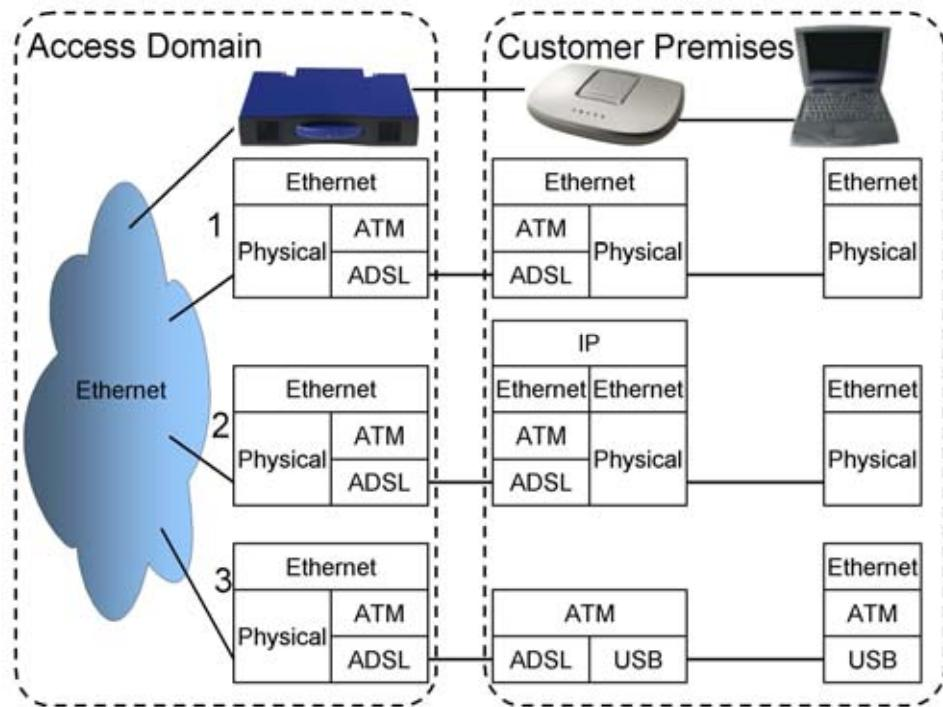
Figure 29 CPE Equipment Protocol Termination
