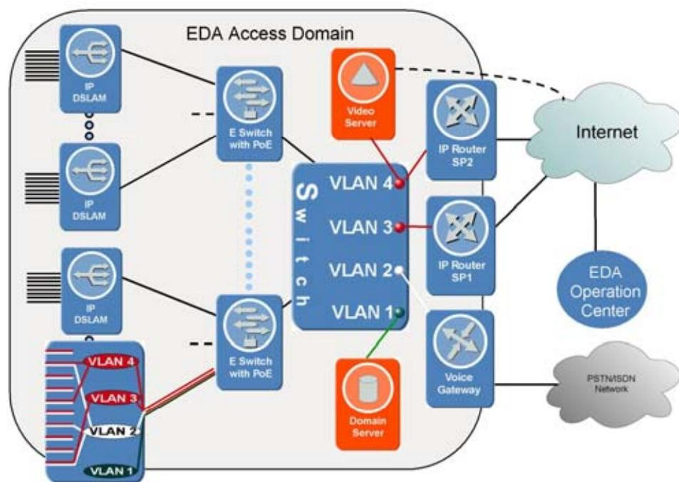
*Figure 62 VLAN-based Scenario with Data Access Services and ToIP*
