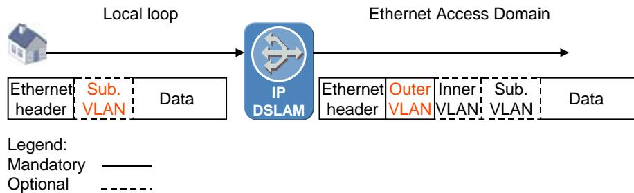
*Figure 35 Using QinQ in EDA*
