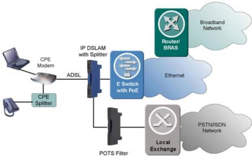
*Figure 50 Base band Solution with External POTS Filter*
