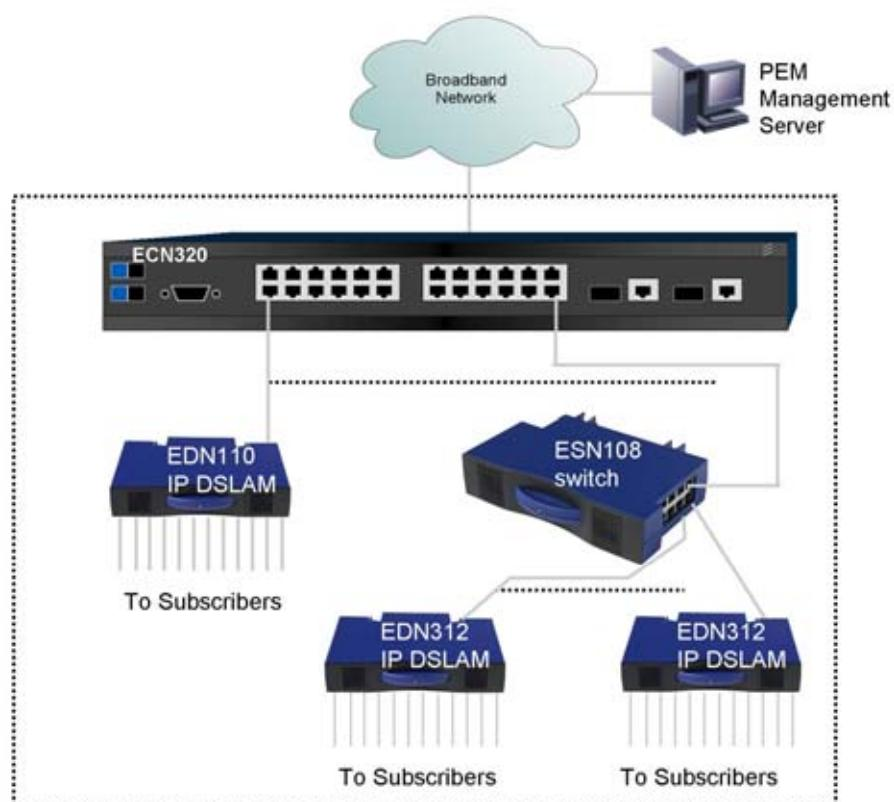
*Figure 8      Example of an EAN*
