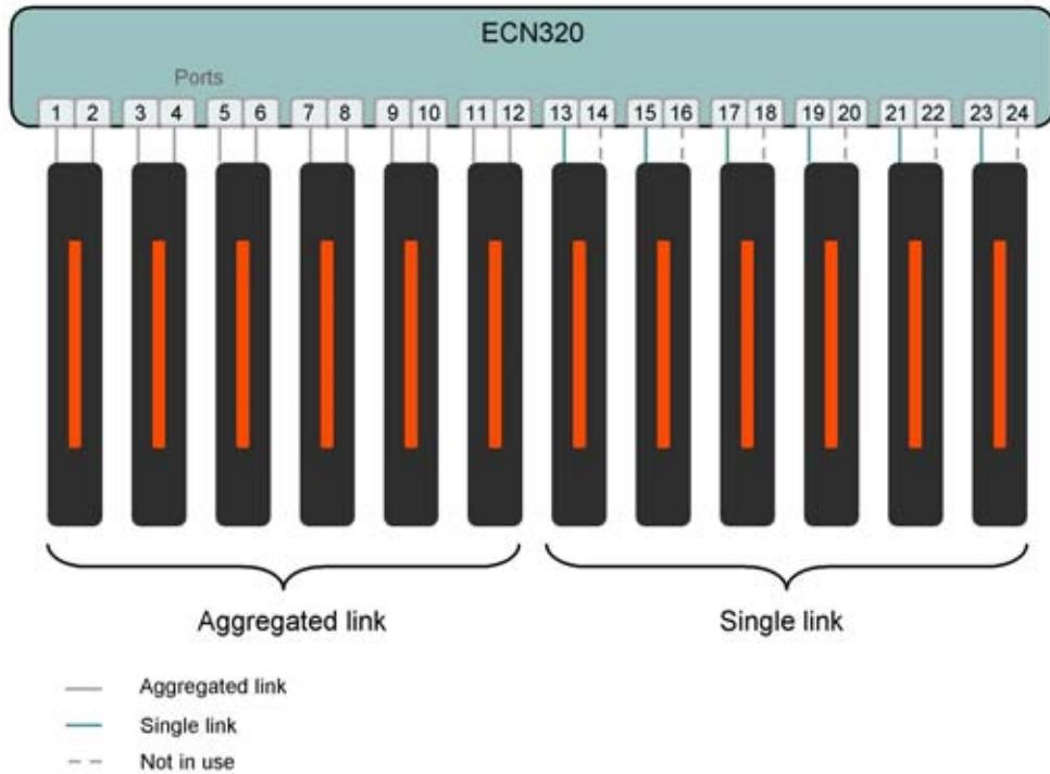
Figure 13 Cabling of Ethernet Cables for Link and PoE Redundancy
