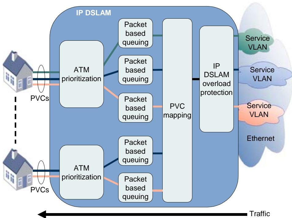
*Figure 42      Downstream QoS Mechanisms*
